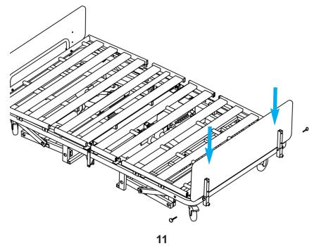
**3d.** Repeat the same process as the footboard for the headboard to complete the assembly.
