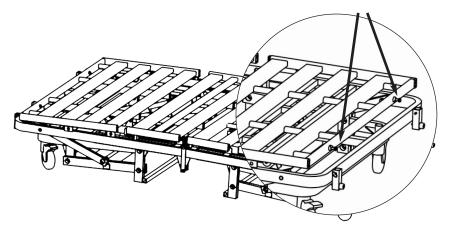
**2b.** Remove the top 2 sets of nuts and bolts on each end of the headframe on the receptacle holders, set the nut and bolts on the side.
