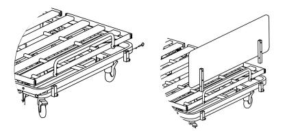
**3c.** Push footboard down all the way until it stops, the holes on the footboard mounting tubes and the holes on the footframe receptacle tubes should line up. Secure the footboard by inserting the two quick-release pins back in the holes. Repeat the same process for the head board.
