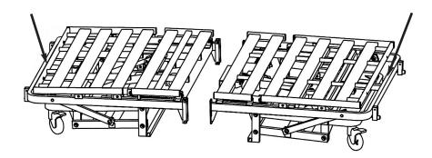
**2a.** Locate the two mattress stop mounting bolts at ends of the bed surface.
