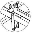
**1c.** Tighten the nuts and bolts on each end with a pair of 13mm wenchs to secure the head and foot frames.
