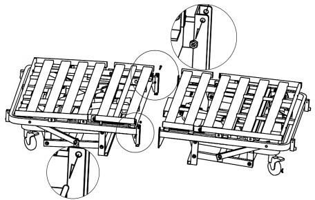
**1b.** Llifting both the tabs and the holders, to bring them together and slowly lower the two sections so as to interlock the tabs and holders. The tab should set into the spacing between the holder and the bolt. Replace the nuts and bolts that were set aside earlier.
