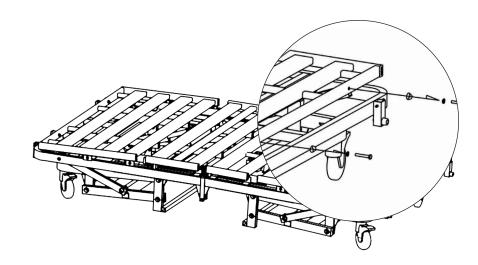
**2c.** Assemble the bolt, washer, and moon shape spacer in order according to the diagram below, and attach the mattress stop bar onto the frame surface.
