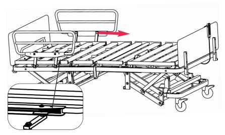
**4c.** Make sure the side with the black release lever faces the foot end of the bed.
