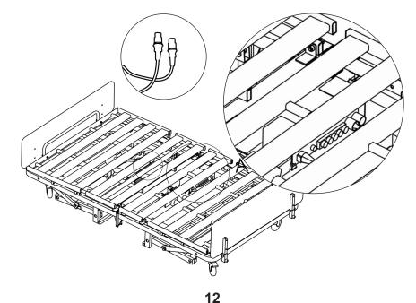
**4a.** The actuator plug are color coded, plug the blue plug into the foot motor receptacles and the yellow into the hi/lo receptacles.
