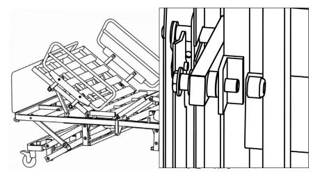
**5d.** Install the bolt and tighten into the holes while holding the nut with your other hand.
