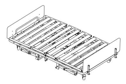
**4.** The two actuators on the foot frame were shipped unplunged, they need to be plug into the junction box for the bed to function. Locate the junction box close to the middle of the bed, on the head-frame side.
