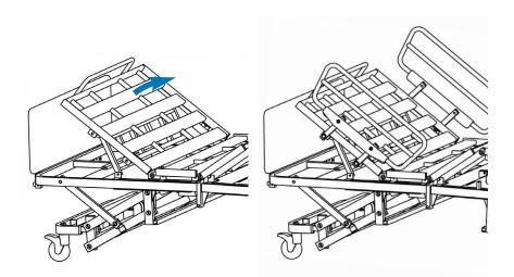
5a. Raise the head frame to expose the holes on top of bed frame.
