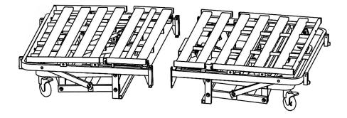
**1a.** Temporarily remove the top 2 sets nut and bolt on each end of the footframe on the receptacle holders, set the nut and bolts on the side.
