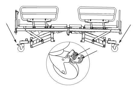
Push down the lower pedal to LOCK the caster wheels Push down the upper pedal to UNLOCK the caster wheels
